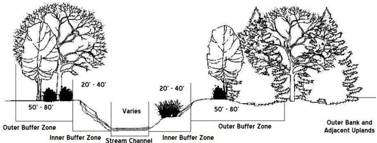
**FIGURE 3 - Cross Section of the Streamside Overlay Zone.** The Streamside Overlay Zone is comprised of a stream channel, an inner buffer zone, an outer buffer zone, and the outer bank. The widths of each of these zones varies based on stream type.
