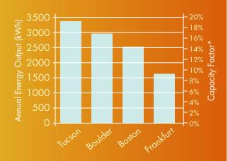
\*Capacity factor: the ratio of the actual output of a power plant over a period of time and its output if it had operated at full capacity the entire time.
