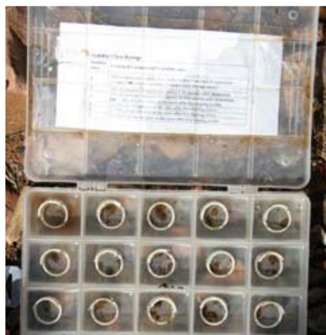
Figure 2. Soil remaining on screen after five dipping cycles.
