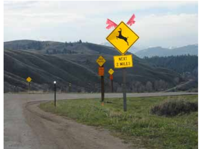
Figure A7: Typical roadside warning sign made nonstandard with the use of flags (© Rob Ament/WTI).
