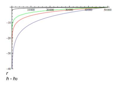
(2) The next figure indicates the effects on drawdown of Q = 1000 (green), 2000 (blue), and 5000 (red) m3/day, also at various distances. Here T = 100 m<sub>2</sub>/day. Drawdown is approximately -2m to -15m at a distance of r = 10 km.
